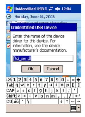
• The device installation is now complete. The installation may be verified using the <u>VCPTest</u> test program available form the <u>Utilities</u> page of the <u>FTDI website</u>.
